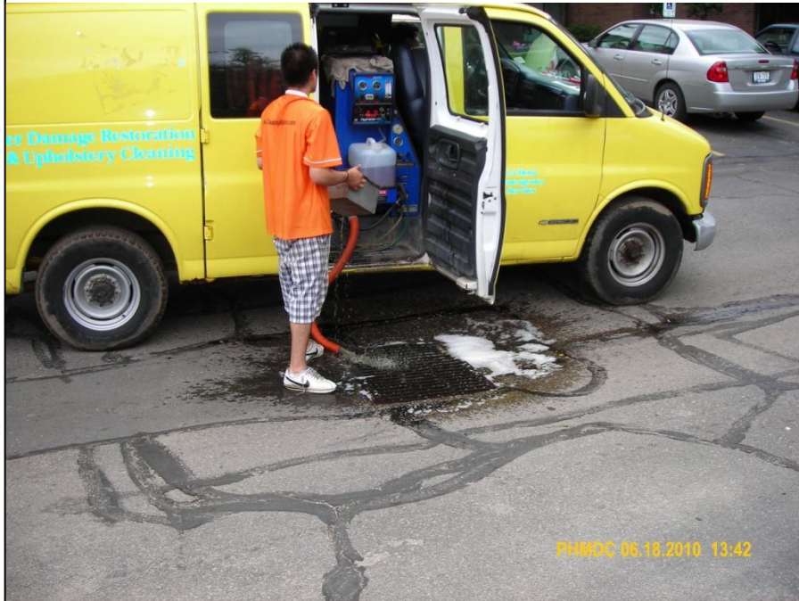
Photo 10: discharge of carpet cleaning wastewater to storm sewer inlet.
